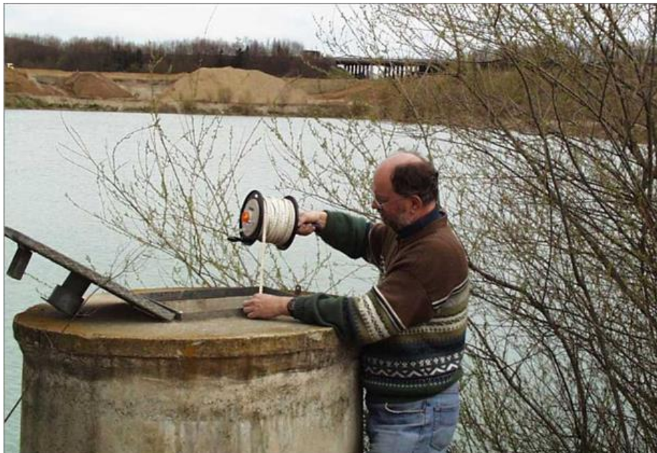
Figure 7: Measurement of the groundwater level before sampling by groundwater level meter, © H. Stadlbauer.
